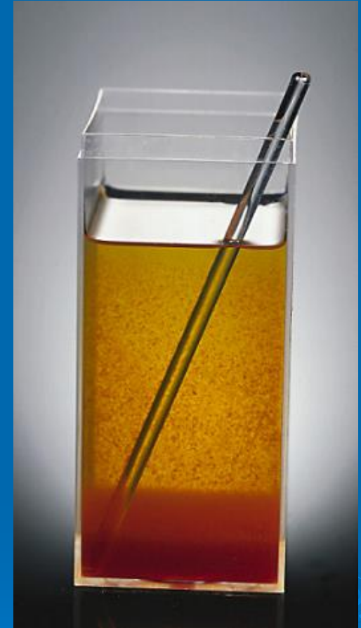
Sol undergoes coagulation upon the addition of \text{Al}_2(\text{SO}_4)_3 solution
